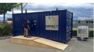
The brewery installation is delivered with a 4-kilowatt electrical generator and accessory valving for heat, hot water, lighting and fire features. Safety features of the system include a 12-volt surplus gas burner safety system, weather protection and secondary containment. The AD process is a 30-day process and the digester has three chambers. Its design is patent-pending and runs as a continuous process. There are no moving parts inside the digester and its designed for a 20-year life cycle.
